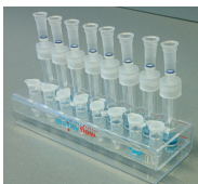
Reference photo: placing the columns and receiving tubes in the Gravity flow rack.
