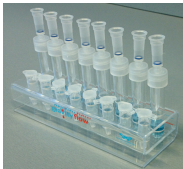
Reference photo: placing the columns and receiving tubes in the Gravity flow rack.
